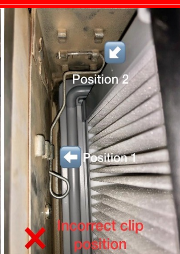
Correct and incorrect positions of the installation frame clip
